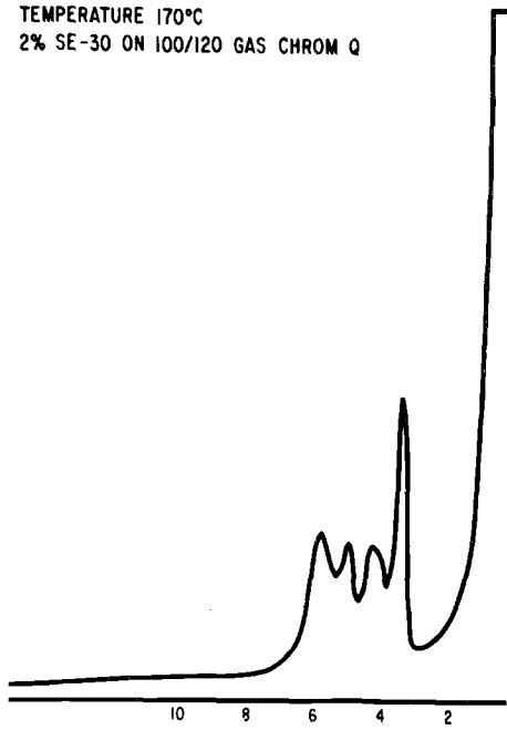
FIG. 3—Separation of sugars using a 2% SE-30 column on gas chrom Q 100/120 mesh at 170 C. Key: a sucrose; b alpha and beta maltose; c alpha lactose; and d beta lactose.
